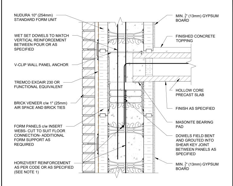
1) FOR OPTIMAL REINFORCEMENT PLACEMENT IN THE NUDURA FORM, SPACING OF HORIZONTAL REINFORCEMENT TO BE SPECIFIED AT 18" (457mm) O.C. AND VERTICAL REINFORCEMENT TO BE SPECIFIED AT MULTIPLES OF 8" (203mm) O.C. REFER TO NUDURA REINFORCEMENT PLACEMENT DETAILS.
